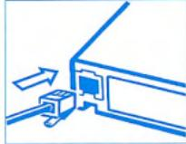
Connect the telephone line to the modem's **TEL IN** (or **IN**) jack.
